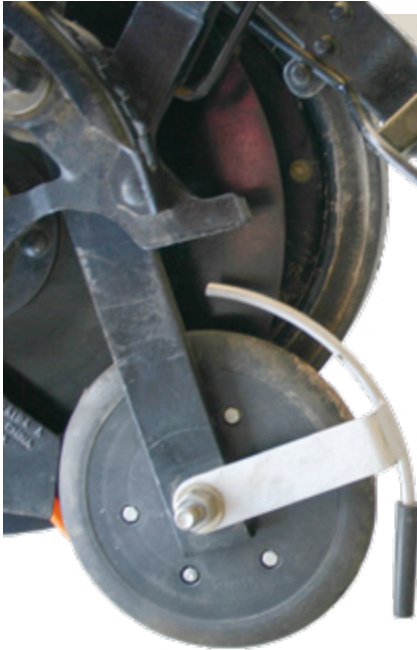
Zipper Max wheel works well on these single press wheel drills
