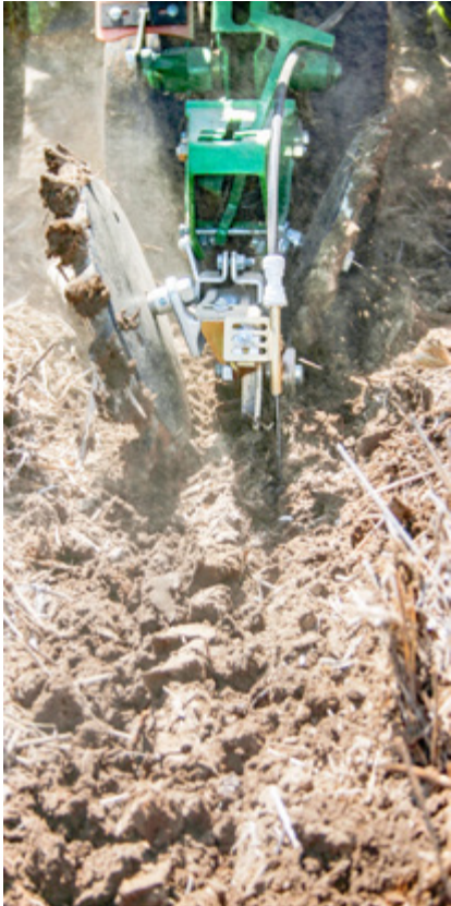
The Zipper closes the furrow in all planting conditions.
