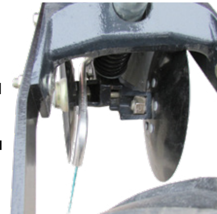
Fertilizer injects directly into the slices cut open by the cover discs
