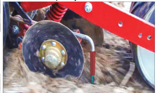
Fertilizer injects directly into the slices cut open by the cover discs
