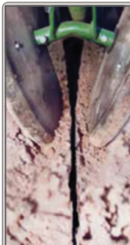
Furrow left open with rubber closing wheels
