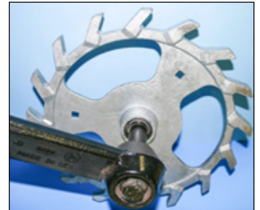
All-cast wheel & stainless steel tube over the press wheel of a John Deere drill
