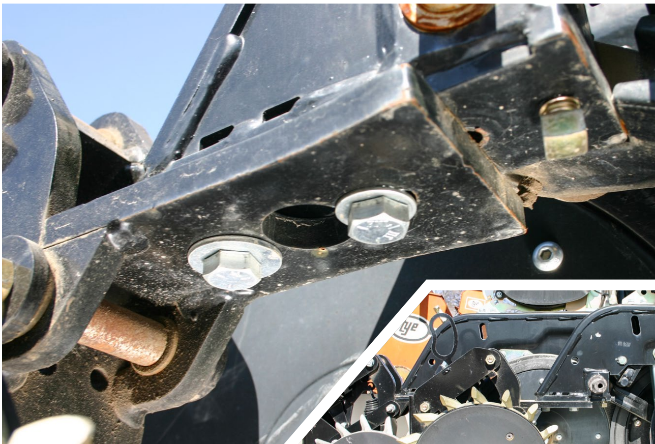
Final assembly of the 4LC with G2 fertilizer arm and Zipper closing wheels
