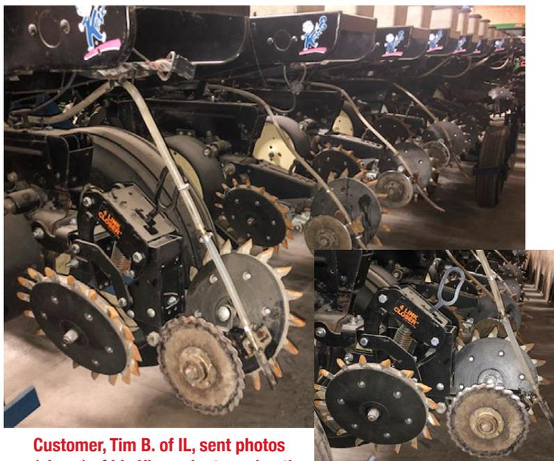
**Customer, Tim B. of IL, sent photos (above) of his Kinze planter using the 4 link closing system on one row in comparison with the factory set-up on the rest of the rows. You can clearly see the improvements made that Tim attributed to not having to run as heavy a down pressure on this row, which meant there was far less sinking and compacting of the soil with this row leading to better emergence.**
