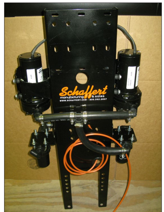
pump system on the tower that mounts in front of the tank
