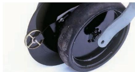
Rotary coulters are recommended in wet or sticky soils.
