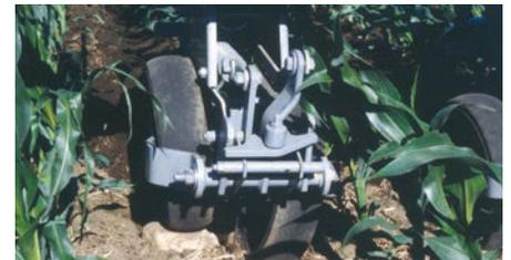
Two 4"x16" heavy duty rubber gauge wheels provide superior flotation while "walking" action ensures precision depth control.
