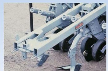
Telescoping trailer hitch provides easy hookup to fertilizer tanks. Hitches are also available for cultivators equipped with lift assist wheels.
