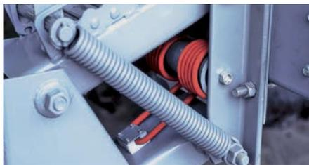
Auxiliary down pressure springs (shown in red) provide extra penetrating power in tractor wheel tracks.
