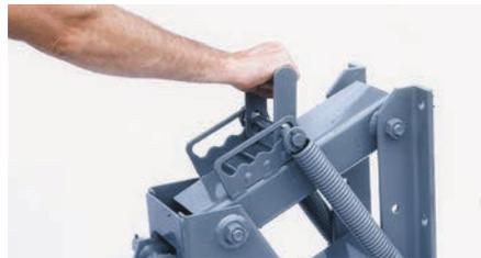
Four-step down pressure adjustment lever for those tough, hard to penetrate soil conditions.
