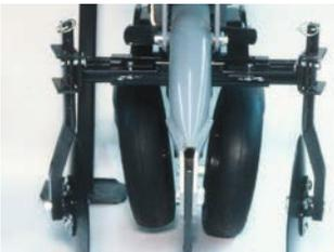
Quick and easy pin adjustments permit 10 horizontal and 14 vertical settings.
