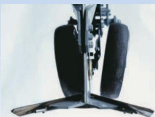
"T" Shaped liquid fertilizer tubes place nutrients on each side of the row for better plant uptake.
