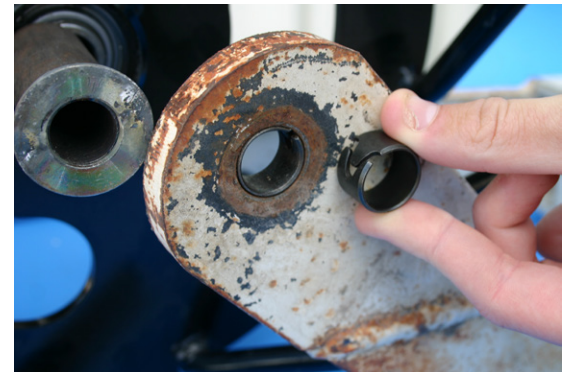
Push Connex bushings into 3/4" bolt holes
