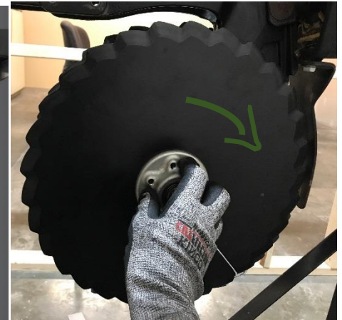
Rotating blade with hub boss
