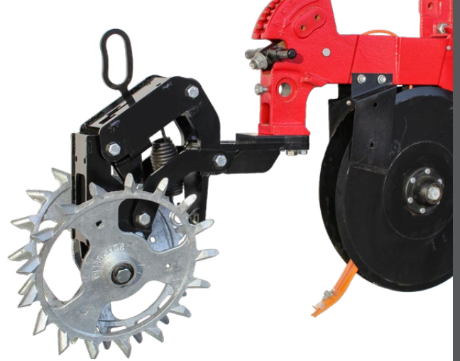
Cast Zippers shown with 4 Link Closer and Rebounder® Seed Cover on a White planter
