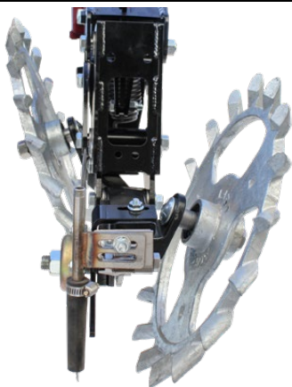
Zippers have been switched around to help eliminate wrapping
